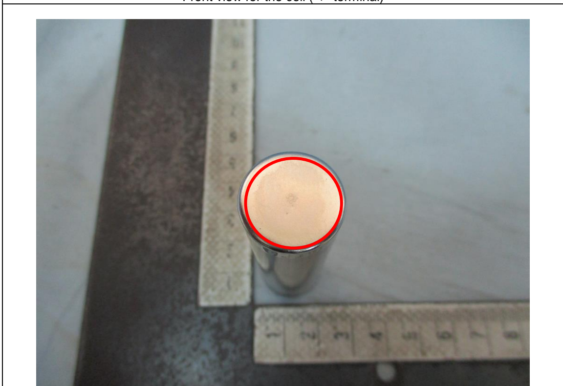
Bottom view for the cell (“-” terminal)
